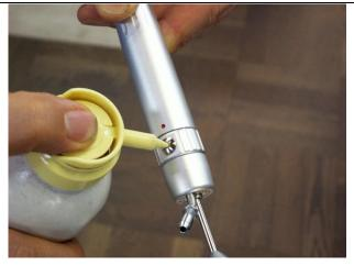
Lubricate by spraying for about 2 seconds as shown in the photo
