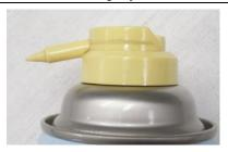
Please prepare a spray nozzle (for cleaning the turbine and chuck) as shown in the photo.
